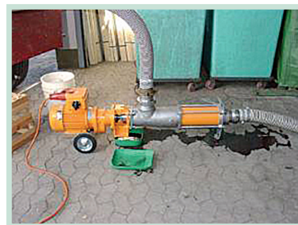
Fig. 63: Mush pump to transport the fermented mush to the press.
