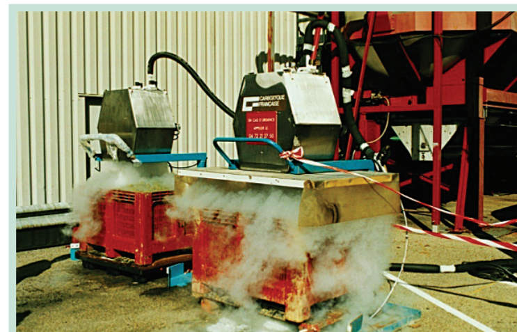
Fig. 64: Technical equipment for cold soaking with dry ice. Production of carbonic snow.
