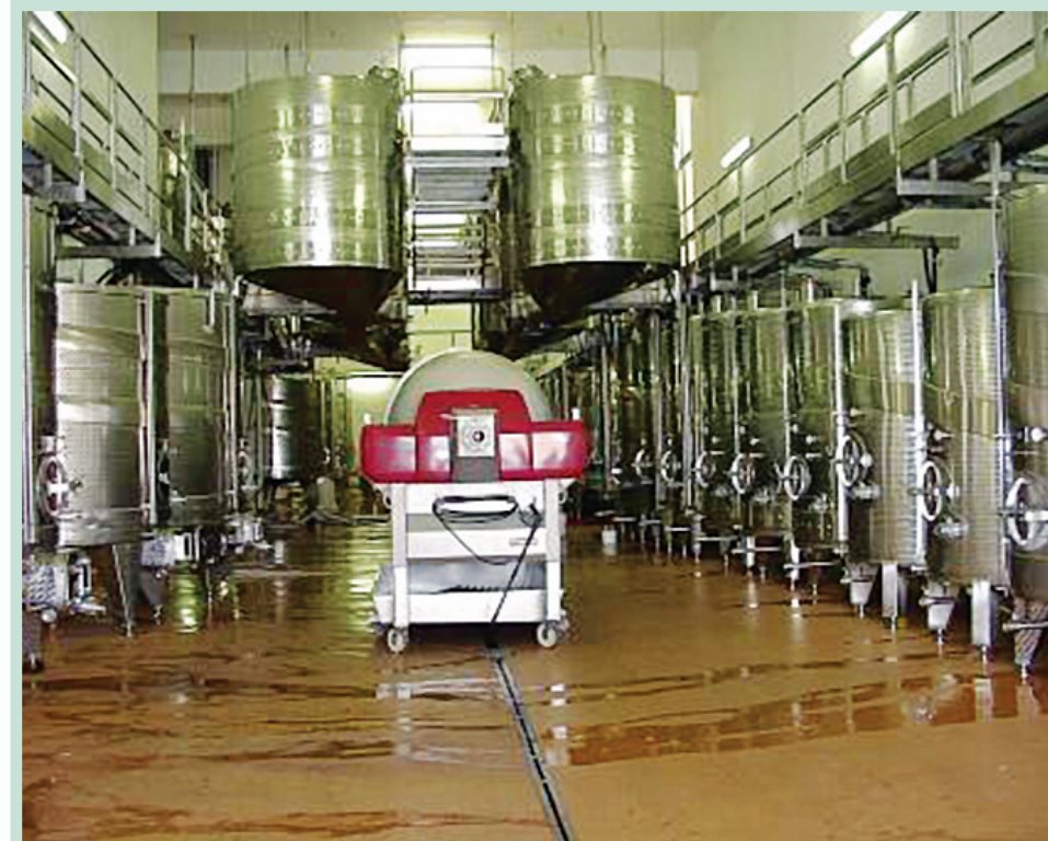
Fig. 62: Red wine fermentation tanks on the top to fill the horizontal tank-press without pumping.
