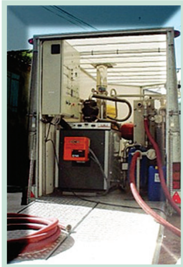
Fig.94: Technical equipment for flash-pasteurisation.
