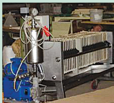
Fig. 45: Grape must Press-Filter and Vacuum Rotation Filter with Cellulose, Diatomaceous earth or perlite
