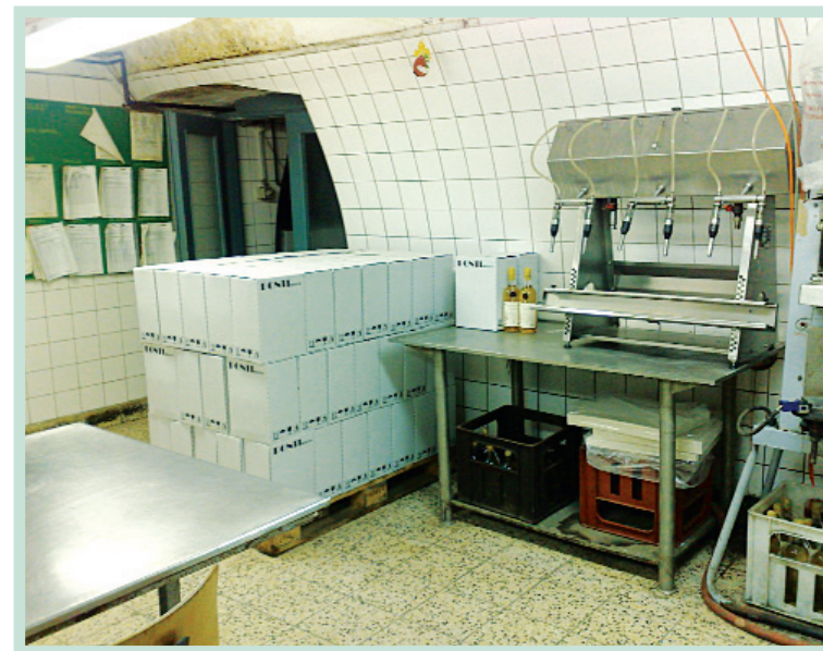
Fig. 78: Bottling machine for a small family winery.
